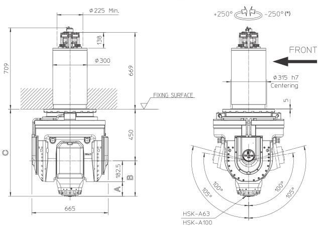
100° PROGRAMMABLE ANGLE 105° MECHANICAL STROKE
