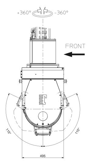
Two axis head with fork structure optimized for heavy 5-axes machines, integrates modules with Technai Direct Drive motors on both axes, and is available with electrospindles up to 12.000 rpm and 40 kW, HSK-A100 tool holder.
