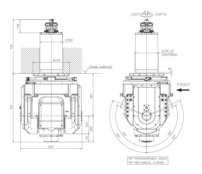
TCH-U 40-50 head declines the concept of universal head for undercut milling operation in the full direct drive version. The goal is achieved by integrating the torque motors of the C and B rotary axes with a powerful electrospindle for the tool actuation. The product is mainly intended for the general mechanical industry and is optimized for milling machines or machining centers with vertical ram (bridge type or gantry machines).
