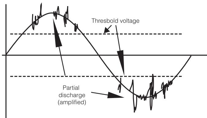
Fig. 1: Partial discharge during dielectric insulation test
