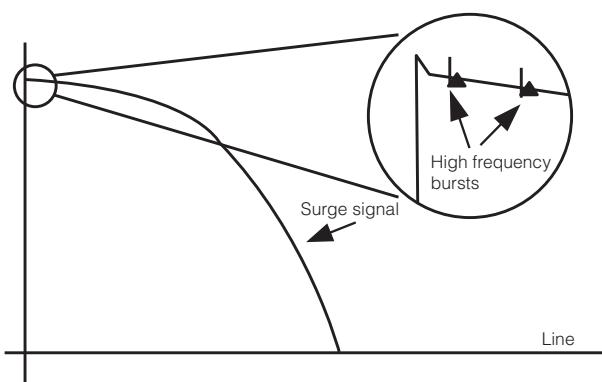
Fig. 2: Partial discharge on surge test signal
